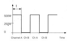
a) Channel A consumes 500 W, while channel B does not consume any power at all. The average power is 250 W. The time is sufficiently short (or the frequency high enough) to avoid the necessity for any time-related limitations.
