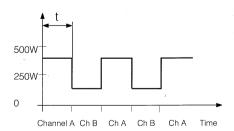
c) This power distribution produces 250 W on average and the frequency is high enough to avoid the necessity for time-related limitations.
