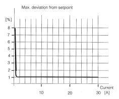
The adjustment accuracy for the resistance depends essentially on the resistance range. In principle, the smaller the resistance, the more precise the adjustment. The second criterion is the applied voltage (the higher the voltage, the more accurate the adjustment).
